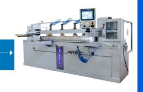
The AMI-C acrylic edge polisher has been designed to polish bevels and angles up to  $60^{\circ}$  thanks to its tilting head (-2° to +60°). The working length of the machine is 2.100 mm and it can polish a maximum thickness of 120 mm.
