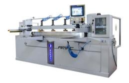
The AMI-C acrylic edge polisher has been designed to polish bevels and angles up to  $60^{\circ}$  thanks to its tilting head (-2° to +60°). The working length of the machine is 3.100 mm and it can polish a maximum thickness of 120 mm.
