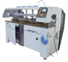
The **AM2-i** acrylic edge polisher has been designed for the machining and polishing of methacrylate PMMA workpieces.
