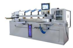
The AMI-C acrylic edge polisher has been designed to polish bevels and angles up to  $60^{\circ}$  thanks to its tilting head (-2° to +60°). The working length of the machine is 2.100 mm and it can polish a maximum thickness of 120 mm.
